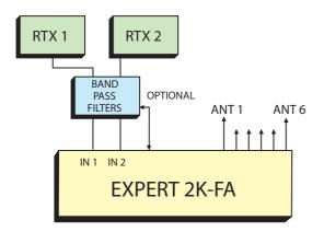
Automatic tuner remotable on the roof (option), you can automatically manage up to 6 antennas with just one coaxial cable feed.
